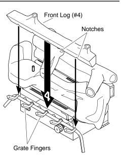
Figure 25 - Installing Front Log (#4)
